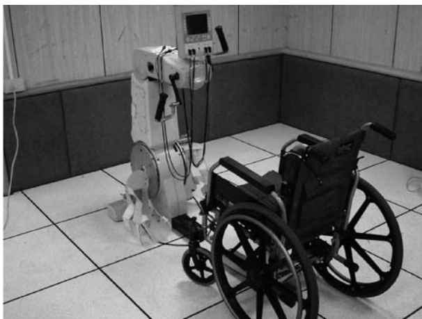
Fig. 1 The FES-cycling ergometer system.
